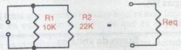
$$R_{eq} = \frac{R_1 \times R_2}{R_1 + R_2} = \frac{10K \times 22K}{10K + 22K} = \frac{220K^2}{32K}$$
